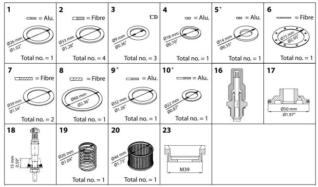
$<sup>^{\</sup>ast}$  The spare part is included in the package but is not used for PM 1 or PM 3..
