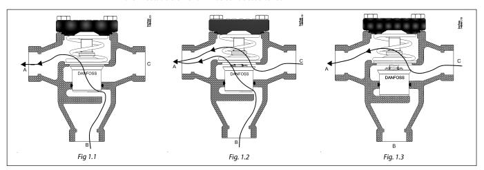
From figure 1, it can be seen how the sleeve on the element is sliding in a vertical movement. The thermostatic element is kept in position by a spring.
