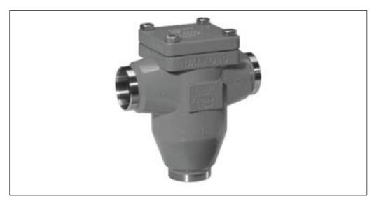
ORV are 3-way industrial valves for maintaining a constant oil temperature in gas compressor systems, by mixing hot and cold oil in the lubricating system of e.g. screw or turbo type compressors.
